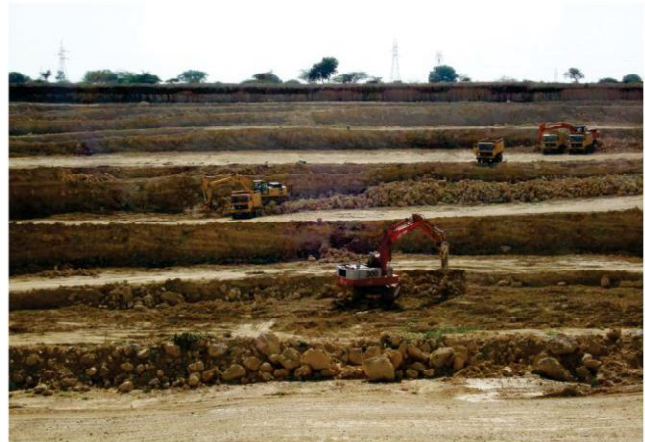
A view of a systematic mining at a Limestone mines belonging to KLK Mines in Tamil Nadu.
