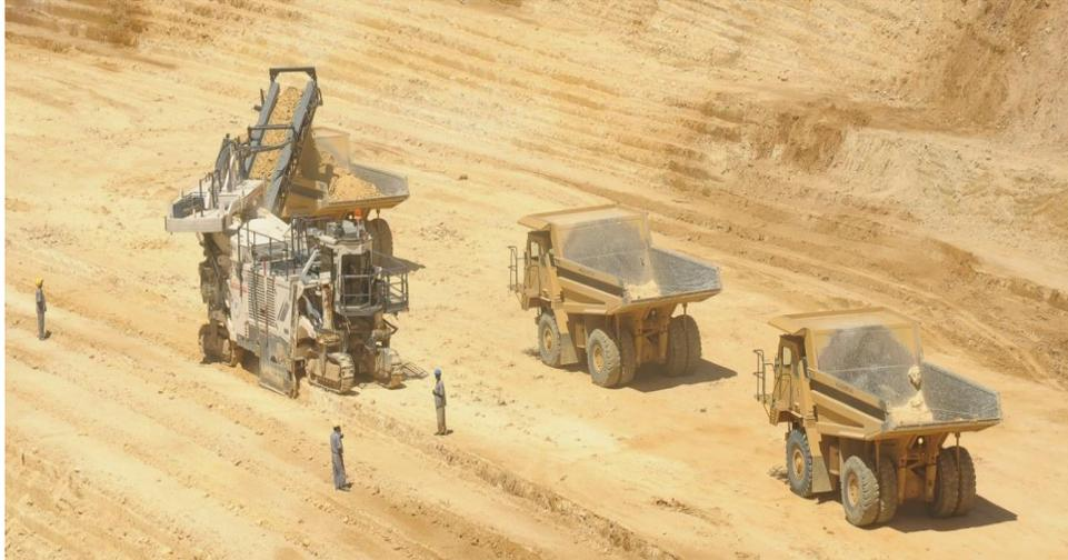
Surface Miner is a machine which cuts the insitu rock in thin vertical or horizontal slices without drilling and blasting, the output size being less than 150 mm. The principle of SM involves cutting the rocks, layer by layer and loading the cut materials into a dumper or conveyor system, which is entirely different from the concept of formation of benches and faces for extraction of mineral by conventional mining.
