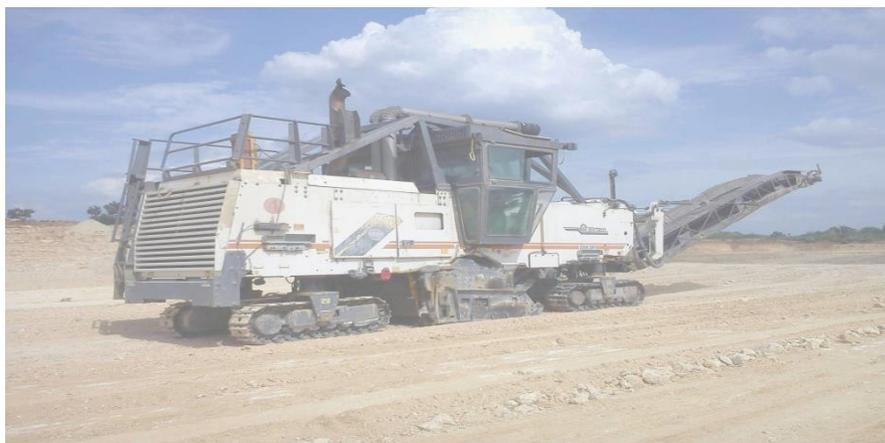
Surface Miner is a machine which cuts the in-situ rock in thin vertical or horizontal slices without drilling and blasting, the output size being less than 150 mm
