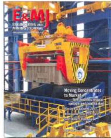
Ausenco designed a containerized system for the Las Bambas mine where custom containers are loaded at the mine and trucked 420 kilometers to a transloading facility. Containers are then placed on trains for the trip to the port where they are discharged to the conventional bulk system for storage and loading onto ships. The final system, commissioned in early 2016, reduced both capital and operating costs by integrating this technology while making use of the existing infrastructure. (Photo: Ausenco)
